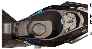
Use the switch lock to unlock the saddle to open the luggage compartment. To lock the saddle, lower it until it clicks. Make sure the saddle is securely locked before riding the scooter. In the luggage compartment you will also find a tool kit
